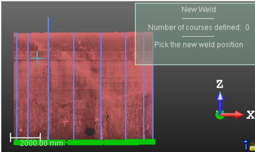
A horizontal line in orange which symbolizes a horizontal weld seam is displayed as illustrated below. Its position along the tank, which is displayed in the information box in the **3D View**, defines its order in regards to the others.
