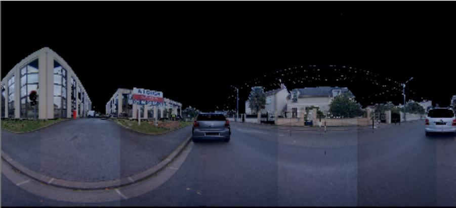
Some color discontinuities between individual images may be visible after coloring the **TZF Scans** (from the **Trimble TX6** and **TX8** instruments). Now in **RealWorks 10.3**, these images are blended so that the quality of the colorization is greatly enhanced:
