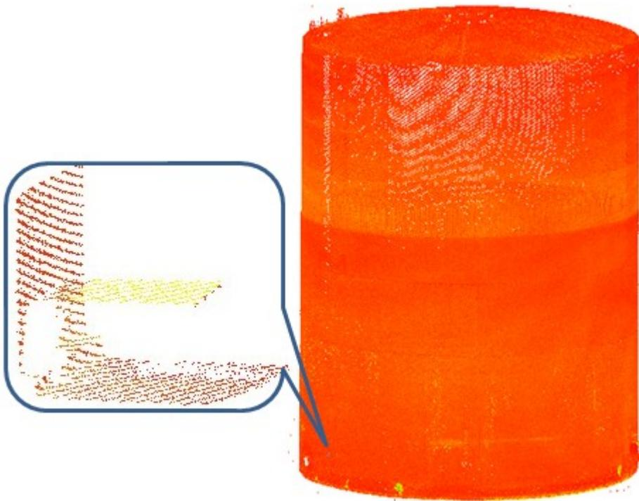
4. Isolate the **Dipping Plate** from the whole set of points by fencing.
