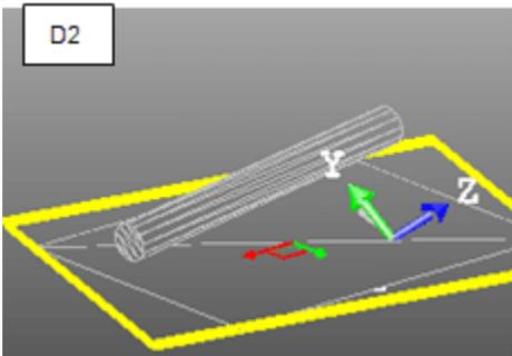
3. Select an axis handle by picking it. It turns yellow. The direction along which you can pan the plane is highlighted in yellow and those (two) for which you cannot are in mauve.
