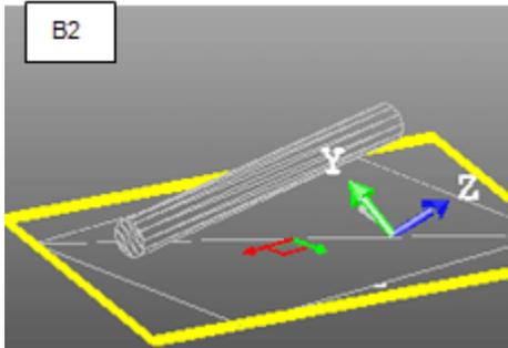
4. Select an axis handle by picking it. It turns yellow. The direction along which you can pan the plane is highlighted in yellow and those (two) for which you cannot are in mauve.
