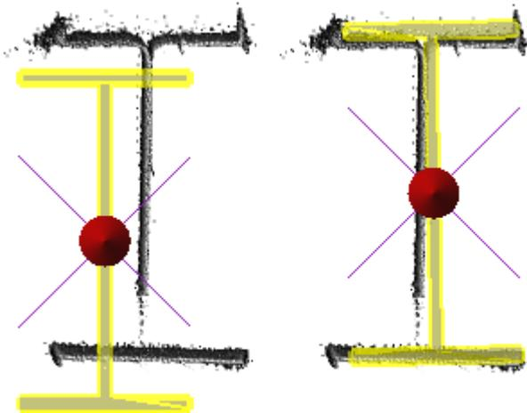
2. Or choose **Adjust** to refit the temporary beam with no constraints. The temporary beam will be moved in any direction to fit the **Cloud Data**.
