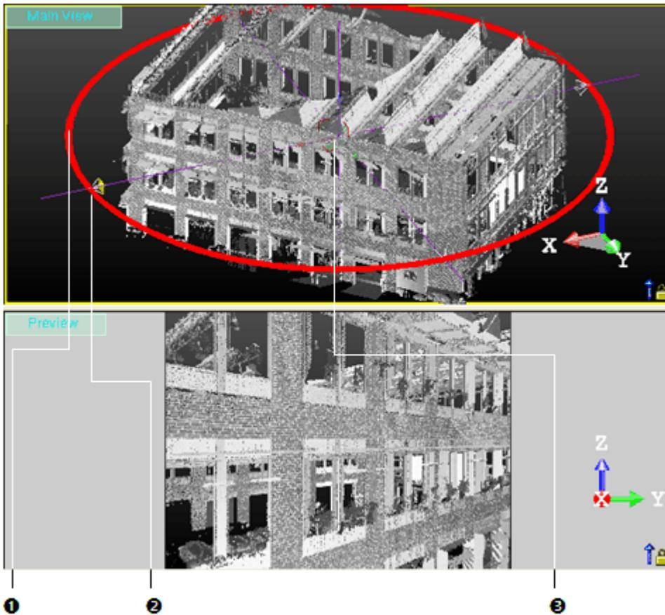
In the **Station-Based** mode, the top 3D viewer displays the global scene with only one keyframe. This keyframe is set at the first station position of the **Project Tree**. The bottom 3D Viewer shows the viewpoint from that keyframe. The **View Inwards/Outwards** button is dimmed.
