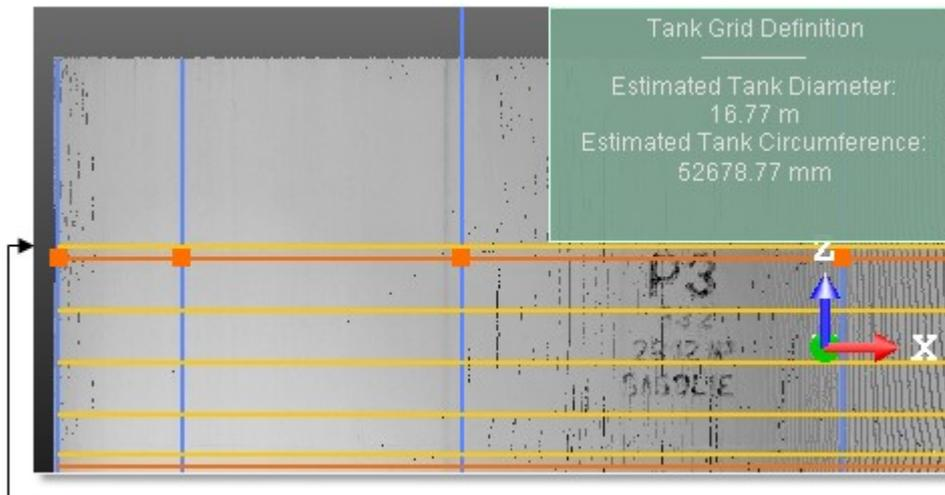
A measurement rule above the bottom weld of a Course
