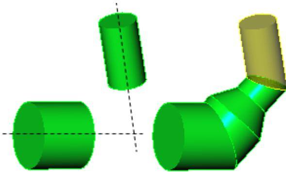
For two cylinders, with aligned axes but not having the same diameter, a regular cone is created in between:
