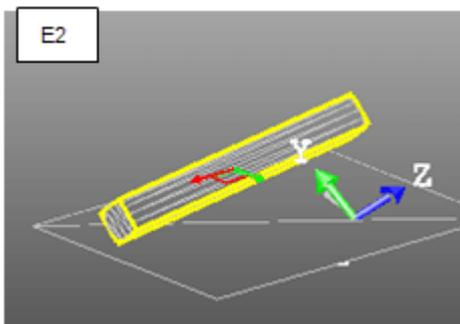
3. Select an axis handle by picking it. It turns yellow. The direction along which you can pan the object is highlighted in yellow and those for which you cannot are in mauve.
