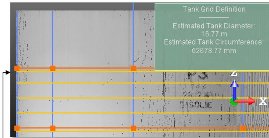
A measurement rule below the top weld of a Course
