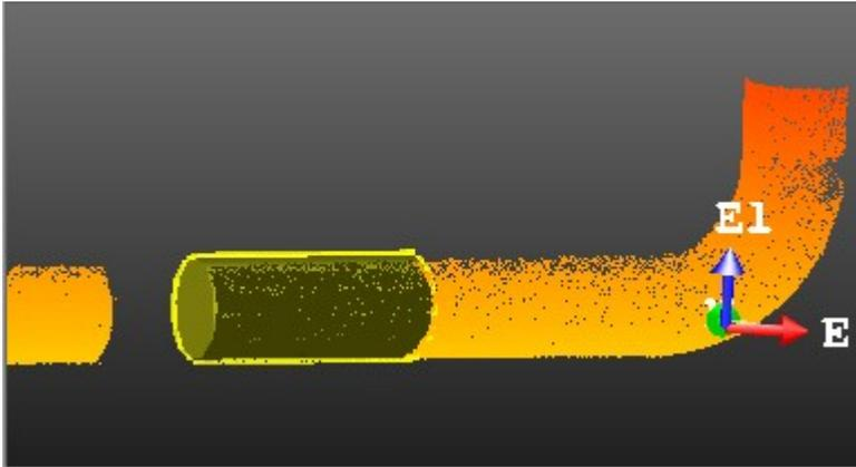
**Note:** An information box at the top right corner of the **3D View** displays the first extracted cylinder parameters like its **Diameter**, the **Number of Points** (used for fitting) and the **Standard Deviation**.
