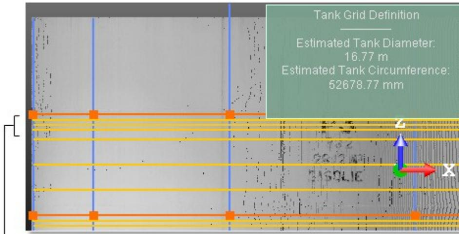
A series of measurement rules below the top weld of a course
