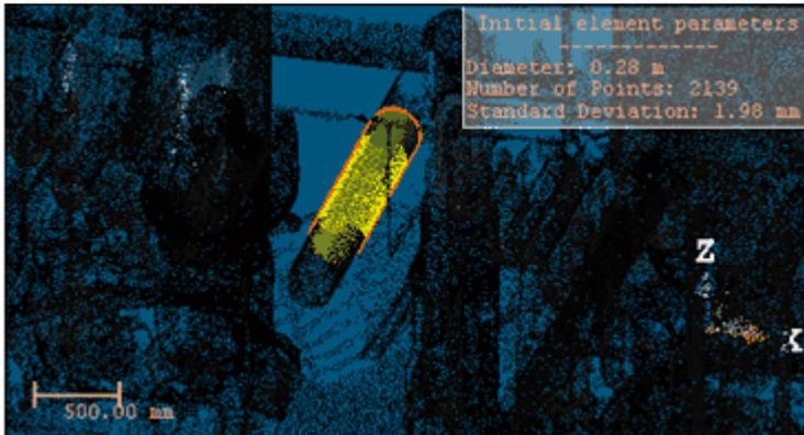
**Note:** An information box at the top right corner of the **3D View** window displays the information related to the picked cylinder like its **Diameter**, **Number of Points** and **Standard Deviation**.
