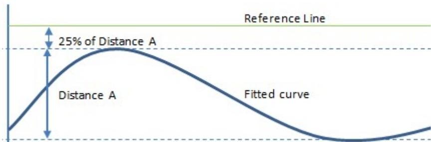
The elevation of this reference line is the elevation of the highest measured point for all the profiles plus 25% of the distance between the highest and the lowest elevations for all the profiles.
