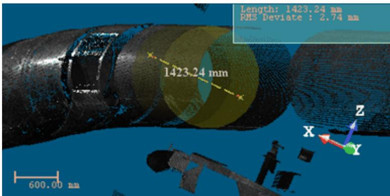
The set of points in the neighborhood of the first picked point is fitted with a cylinder and its diameter is measured and displayed.
