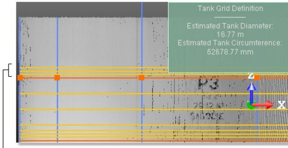
A series of measurement rules above the bottom weld of a course
