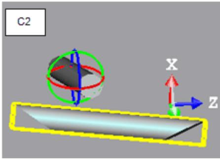
5. Select a ring handle by picking it. It turns yellow. An axis passing the center of that ring handle and perpendicular to it appears. This axis has the color of the selected ring handle.
