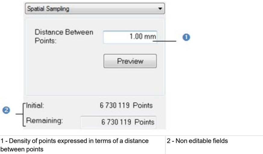
This dialog displays two numbers: **Initial** and **Remaining**. The **Initial** number is the total number of points before sampling. The **Remaining** number corresponds to the number of points after sampling. The unit of measurement is set by default in millimeters; but you can change it when necessary in **Preferences**.
