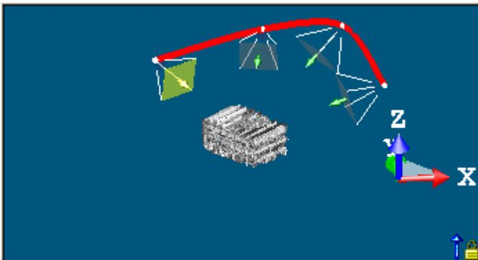
In the **Walkthrough** navigation mode, a new keyframe is added in the top 3D viewer at the same position as the previous keyframe but with a different direction if you tilt or look at a direction. A red curve path links this new keyframe to the previous keyframe if you pan or walk through the scene.
