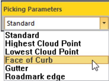
A **Face of Curb Point** is the most external (i.e. closest to the road) and highest point on the sidewalk. It always corresponds to a real (acquired) 3D point in the point cloud.
