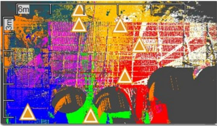
The **Preview** is an **Ortho-Image** of low resolution which is about 0.1 megapixels. The **Ortho-Image**, which is split into a set of small pieces of **Ortho-Image**, is of high resolution which cannot exceed 10 megapixels. Each split **Ortho-Image** is named as follows **ImageX\_Line Index\_Colum Index**. It has a size (W x H) in pixels which is about 500 x 500 pixels.
