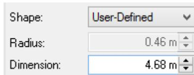
When you change the value in the **Dimension** field, its shape does not lengthen or shorten as for the predefined shapes. You will only see the hoop(s) moving as well as the 3D plane.
