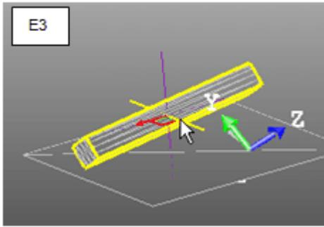
5. Select the plane handle by picking it. It turns yellow. The directions (two) along which you can pan the object are highlighted in yellow and the one for which you cannot is in mauve.
