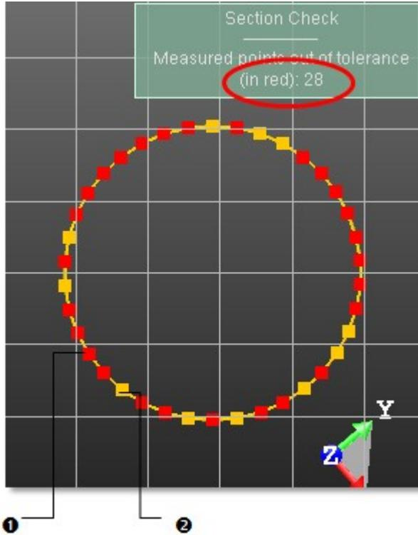
1 - A measurement point out of the defined Tolerance
