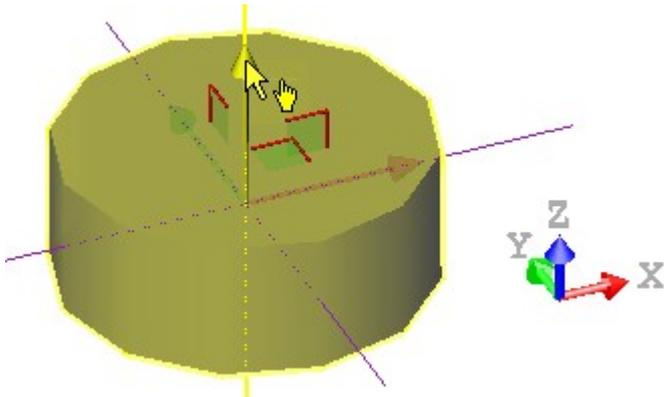
5. Select a plane handle by picking it. It turns yellow. The directions (two) along which you can pan the selection are highlighted in yellow and the one for which you cannot is in mauve.
