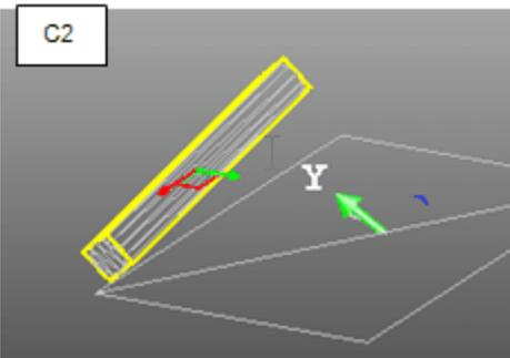
4. Select an axis handle by picking it. It turns yellow. The direction along which you can pan the object is highlighted in yellow and those for which you cannot are in mauve.
