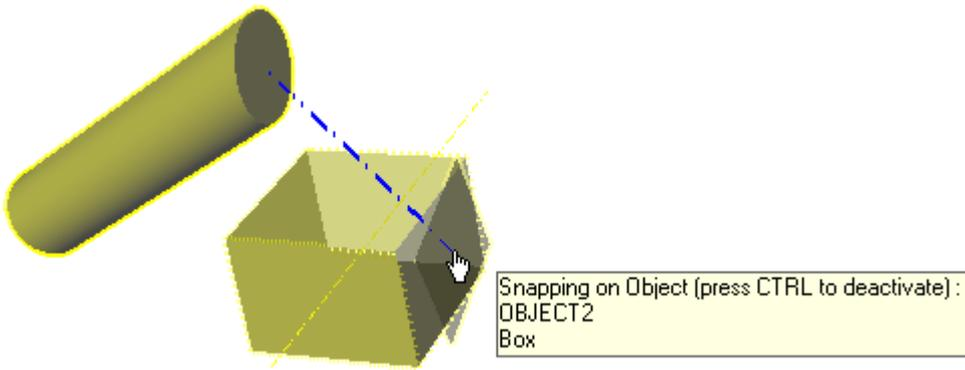
**Note:** If you don't want to snap on any face, press the **CTRL** key while dragging the handle.
