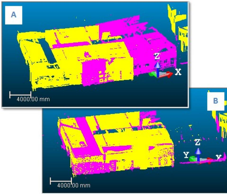
A - Common parts of the clouds are not yet superimposed B - Common parts of the clouds are superimposed
