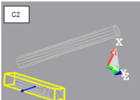
6. Select the position manipulator. It turns yellow. The direction along which you can pan the second object is in yellow and those (two) for which you cannot are in mauve.
