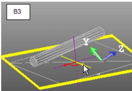
6. Select the plane handle by picking it. It turns yellow. The directions (two) along which you can pan the object are highlighted in yellow and the one for which you cannot is in mauve.
