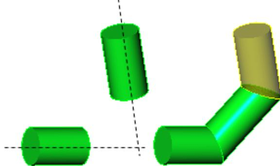
For two cylinders, not secant in axes and not having the same diameter, two connected cylinders and one regular cone are created in between:
