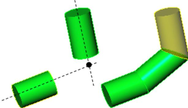
For two cylinders, not secant in axes and having the same diameter, a connected cylinder is created in between:
