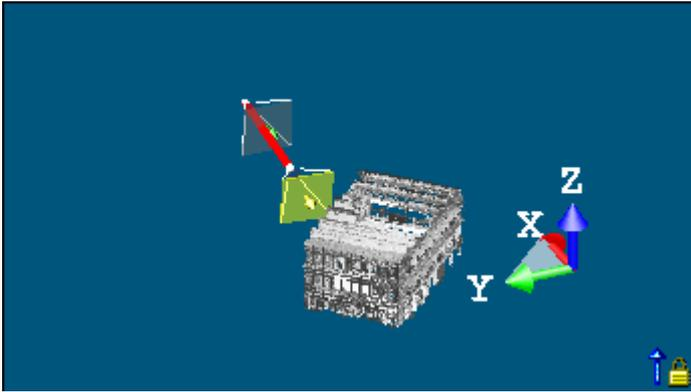
In the **Station-Based** navigation mode, a new keyframe is added in the top 3D viewer at the same position as the previous keyframe but with a different orientation if you rotate (or zoom) or at the second station position if you jump to the second station. There is no red curve path linking this new keyframe to the initial keyframe.
