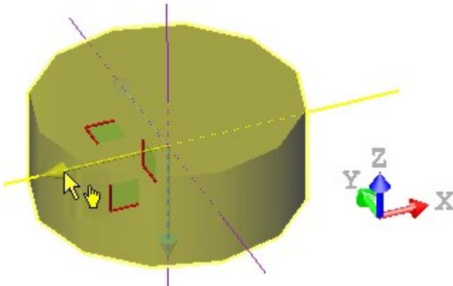
5. Select a plane handle by picking it. It turns to yellow. The directions (two) along which you can pan the selection are highlighted in yellow and the one for which you cannot is in mauve.
